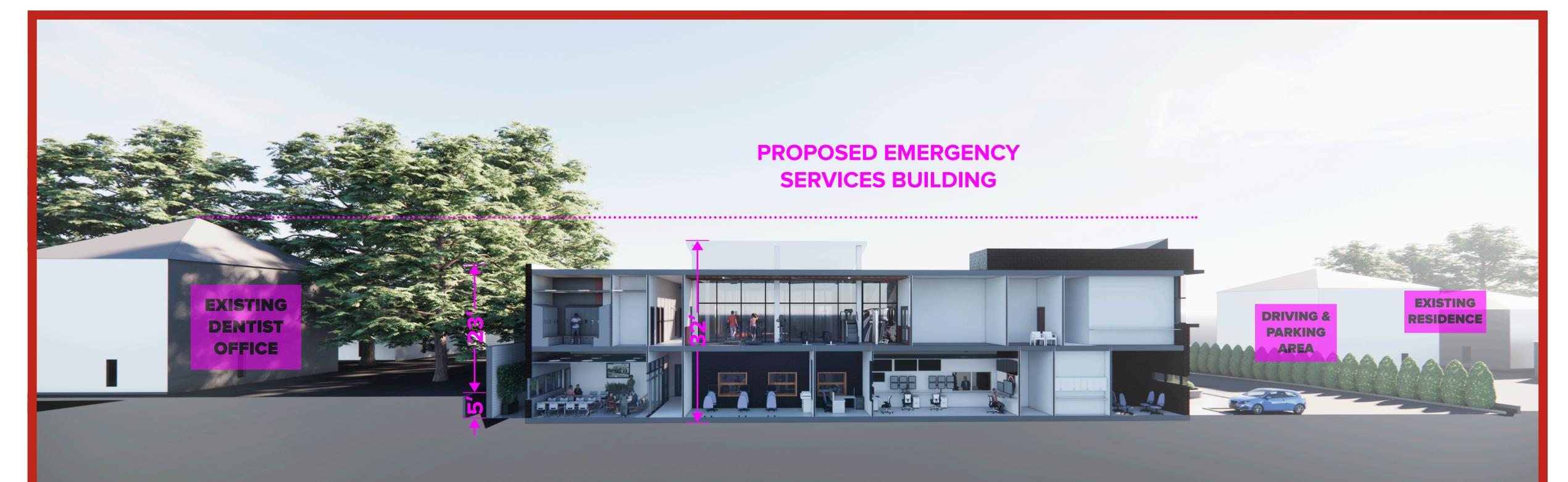
The section above shows the relationship to and defines the impact on the adjacent properties. With the site being an average of 5' lower and with a building height of 33' at the tallest projection, it is lower than the adjacent residence to the West. It should be noted that the average height of the building across the site is 28'.
